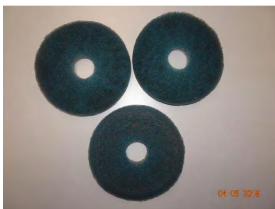
Abbildung 211: WNG ID 920: Zuluftfilter
