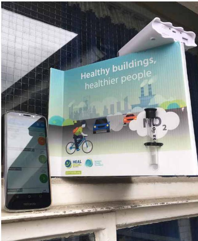
► Air beam monitor and NO<sub>2</sub> tubes to measure air pollutants. | © Sustrans |
