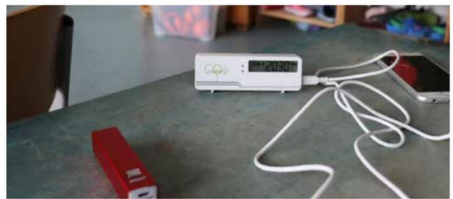
► A mini CO<sub>2</sub> monitor was used which contains a traffic light system for classifying the indoor CO<sub>2</sub> concentration. | © HEAL |
