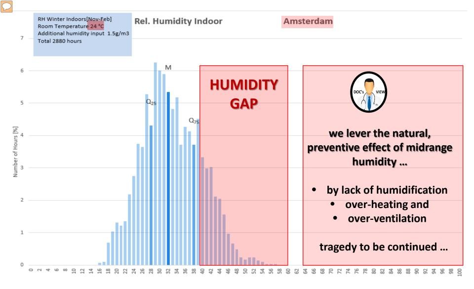
Histogram shows calculated frequency distribution of RH from Nov. to Feb. in Dutch buildings Assumptions: temperature 24 °C, ventilation 29 m<sup>3</sup> ODA/person/hour  $\rightarrow$  humidity input by occupants 1,5 g/m<sup>3</sup> ODA.
