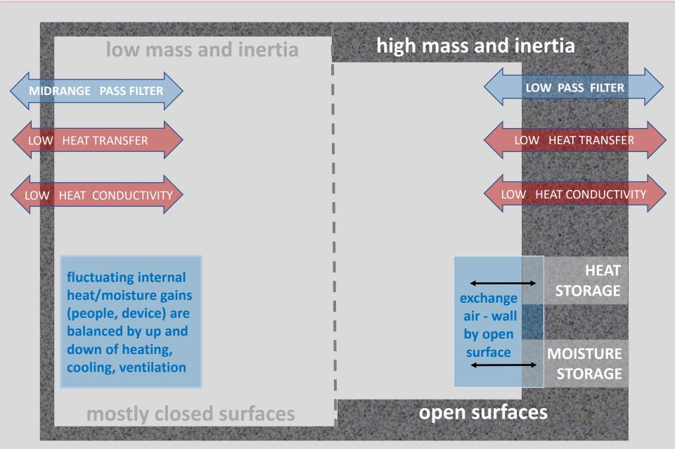
Two energy efficient building concepts lightweight, high tech – low tech, mass/inertia
