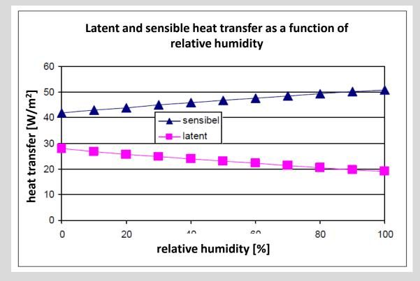
Heat transfer of humans in Watt/m<sup>2</sup> body surface. In increasing humidity and consistent comfort feeling, the ratio between latent and sensible heat transfer shifts. Assumptions: 1,2 met, 1,4 clo, V<sub>air</sub> = 0,15
